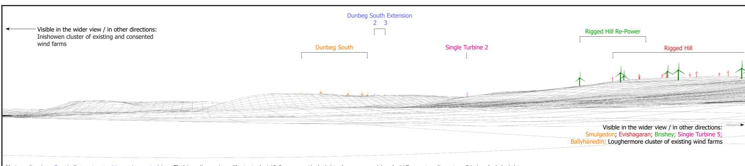
Notes: Dunbeg South Extension turbines shown in blue. Turbine dimensions illustrated: 149.9 m max. tip height above ground level; 117 m rotor diameter; 91.4 m hub height Where present in view: Existing wind farms in red; Consented wind farms in orange; Proposed wind farms in green; Single turbines in pink / in the baseline photography.
