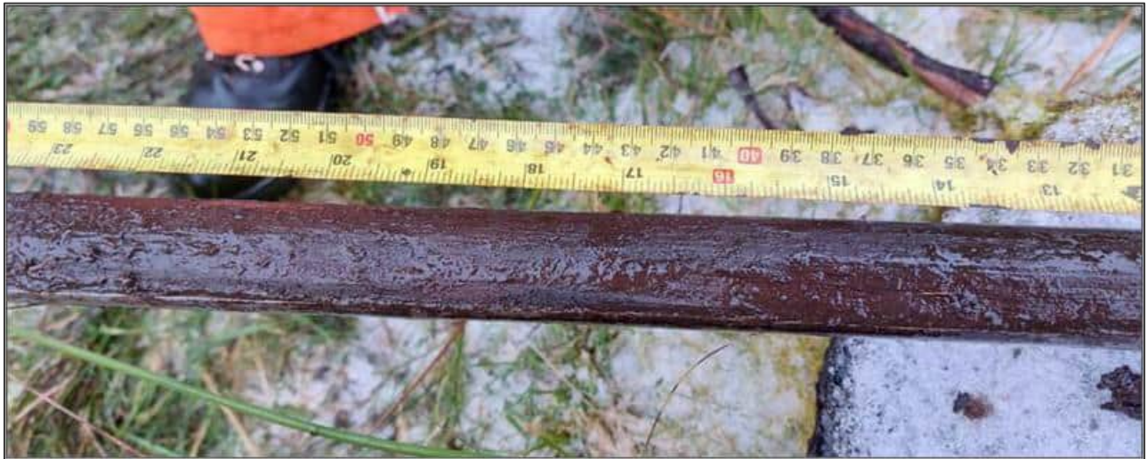
Figure B. 5: Peat core photograph from peat probe position 108 showing firm dark brown plastic pseudo fibrous peat (H7/B2)
