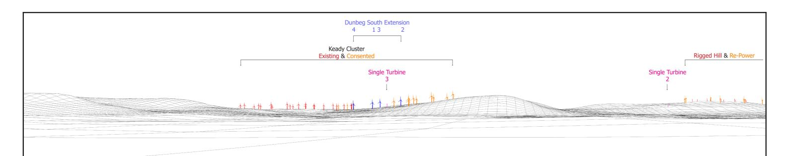
Notes: Dunbeg South Extension turbines shown in blue. Turbine dimensions illustrated: 149.9 m max. tip height above ground level; 117 m rotor diameter; 91.4 m hub height Where present in view: Existing wind farms in red; Consented wind farms in orange; Proposed wind farms in green; Single turbines in pink / in the baseline photography.
